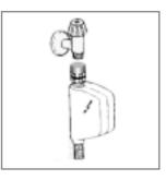
After turning off the water tap, unscrew the end of the water supply hose, remove the filter and clean it carefully under running water. Then, return the filter to its place and tighten the water supply hose back into position.
